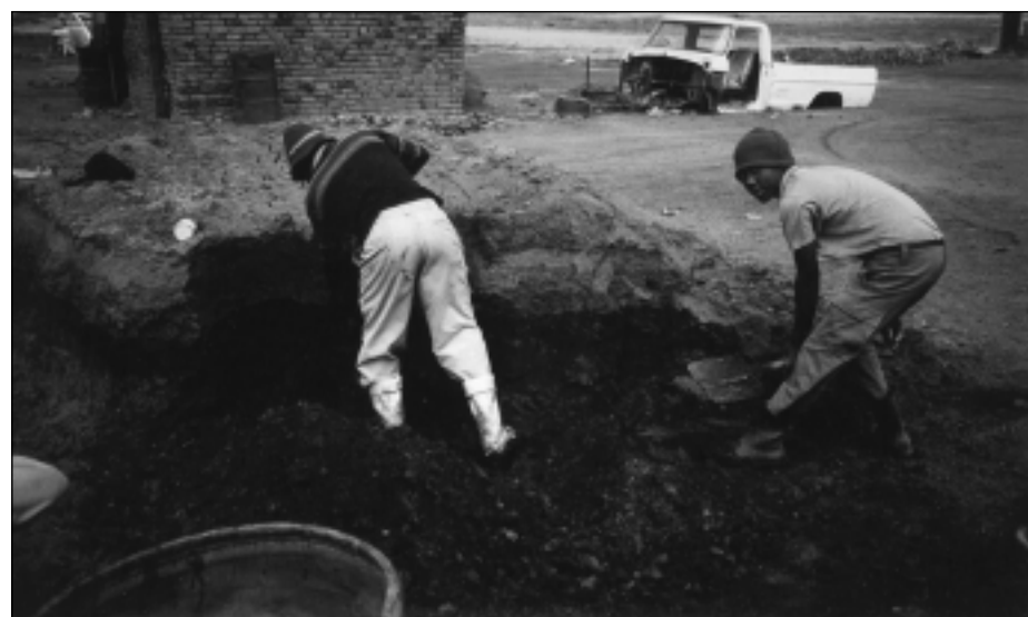
Fig. 11: Manual mixing of saw and coal dust with clay
